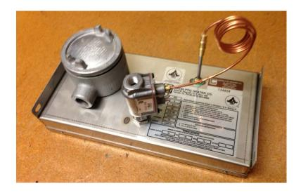
Heaters with a CGA Configuration include the valve, thermocouple, explosion proof junction boxes and low pressure fuel gas regulator. This configuration is approved by CSA for Class I, Div I or II, Group D atmospheres.
