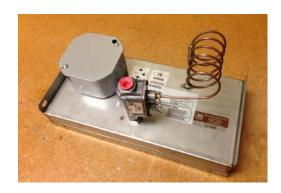
The SFT Configuration includes the valve and thermocouple. This is recommended for applications that are indoors, using propane for fuel or require a certification label. This configuration of heater is approved by Factory Mutual for Class I, Div II, Group D. It includes a plain electric junction box.
