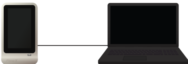
Figure 9-1 Direct Ethernet connection without switch
