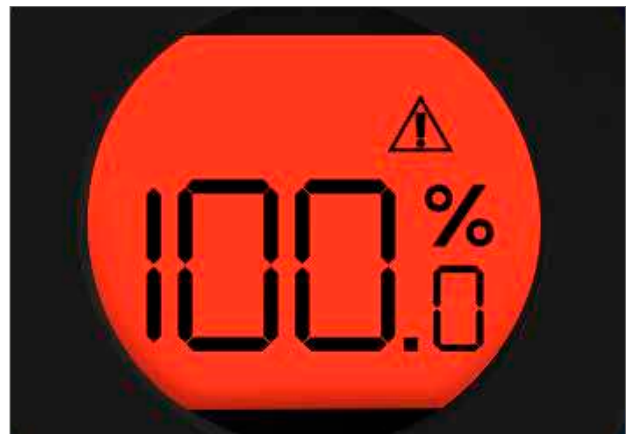
Fig 4.7 Actuator flashes Red and White alternatively when power failure occurs
