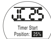
Timer Set to Start Pulsing when Closing Valve Reaches 25% Open
