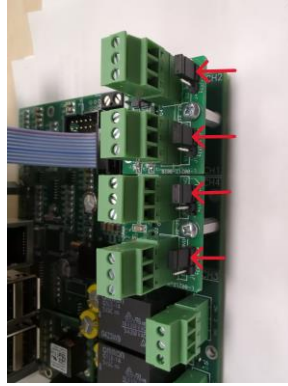
FIGURE (4.C.5)- Choosing internal or external powering of AOs
