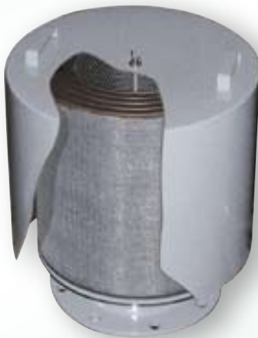
A B70 filter shown cut away to illustrate an optional "K200" woven wire mesh filter element inside. Like K5 elements, K200 elements can be used dry for high flow services (K200 dry is 750µ), or when wetted with ordinary motor oil K200 can perform at down to 10µ retention in normal installation conditions. See page 30 for a list of optional filter media and connection style alternatives for these filters.
