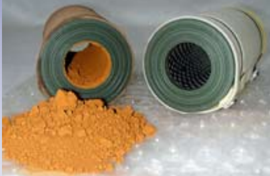
Before and after, shows one of our coalescing elements and the pipe scale and dirt it filtered out of an air line. (Coalescing flow is inside to outside) At right is a new element ready to go into service
