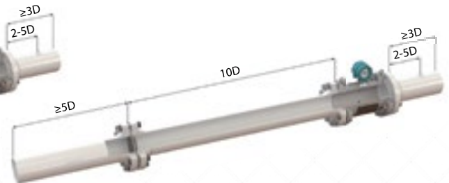
CONFIGURATION 3 Conservative configuration with flow conditioner
